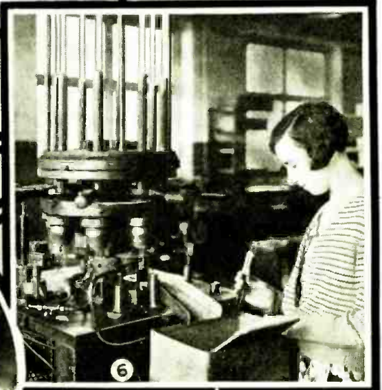
(6) Automatic Flare Machine —Long lengths of glass tubing are placed in the revolving chucks which are shown at the top of this machine. These chucks feed the glass tube, at a predetermined, desired length, into a number of gas flames. There are eight sets of gas flames which the tube passes through from the time the operation starts until the flare is finished. Each different position is accompanied by an increase of temperature of the flame acting upon the glass tubing as the process develops. At the position shown directly before the operator is a revolving steel flare cutting disc.
