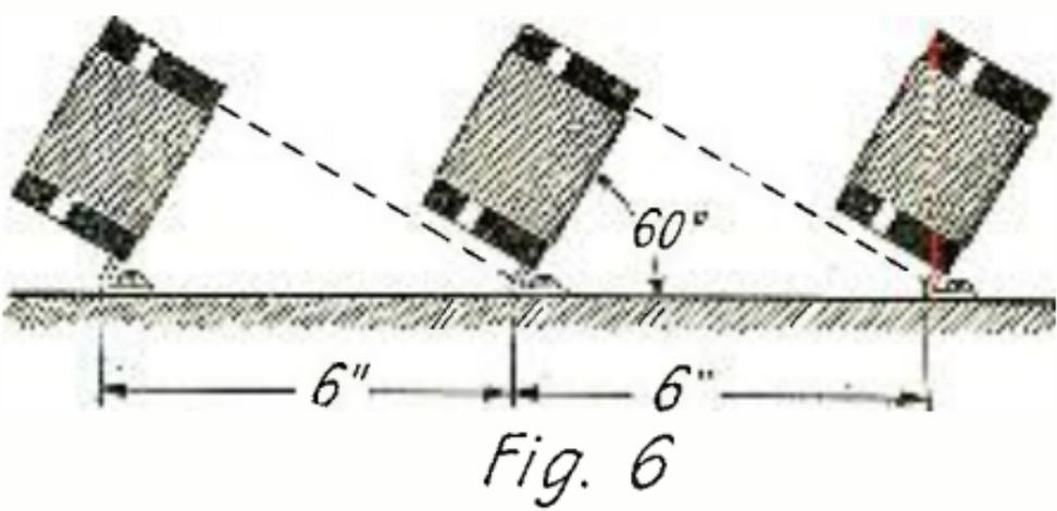
It Is Important That the Radio Frequency Transformers Be Mounted as Shown in the Above Illustration.
