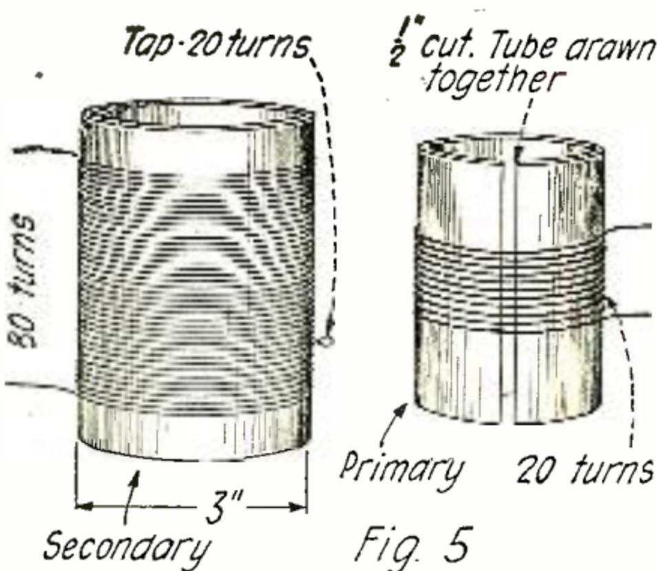
Constructional Details of the Primary and Secondary Coils of the Neutroformers
