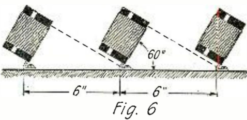
It Is Important That the Radio Frequency Transformers Be Mounted as Shown in the Above Illustration.
